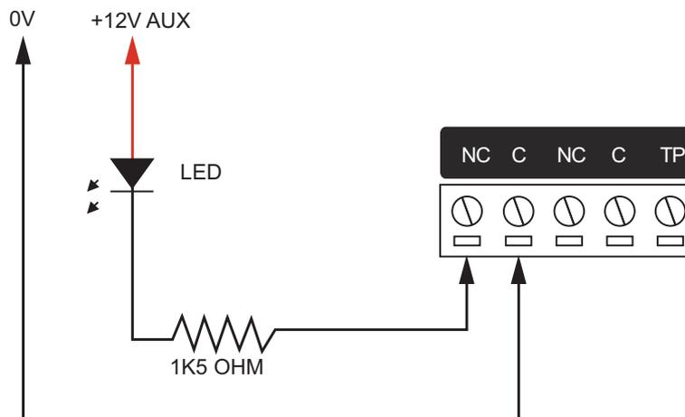
**Warning:** Switching inductive loads that can produce high back EMF voltages or large voltage induced spikes can cause the module to behave unexpectedly and should be avoided. A suitable isolation circuit must be installed between the relay contacts of the module and the inductive load.
