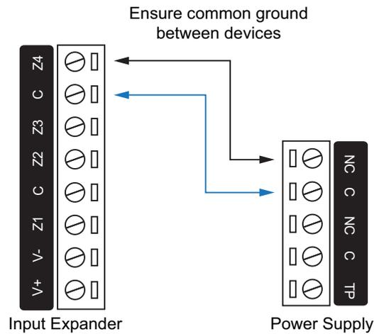
This output is suited for connection to an input on a Protege module with spare inputs available so that the Power Supply AC status can be externally monitored. The connection example above shows monitoring of the AC Status set up in conjunction with a Protege Input Expander.
