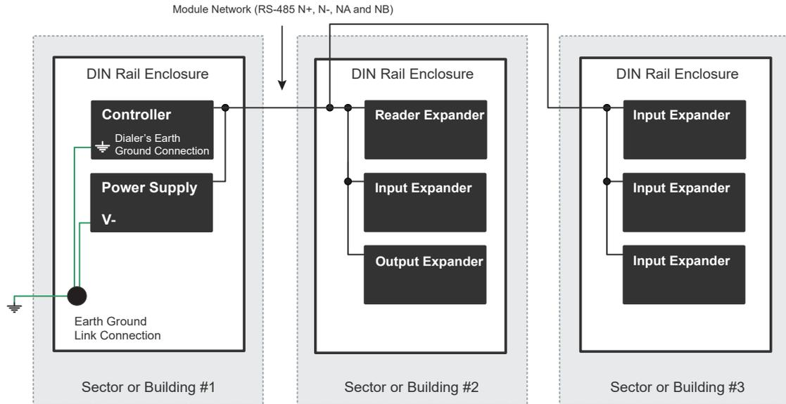
Note that the DIN Rail enclosure earth terminal is connected to the power supply V- terminal.
