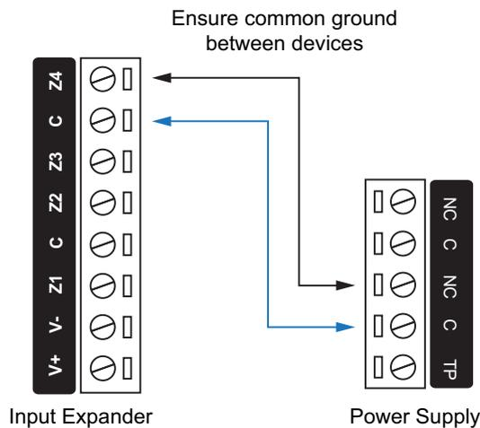
This output is suited for connection to an input on the Protege System for early detection of complete power failure. The connection example above shows monitoring of the Battery Status set up in conjunction with an Input Expander.
