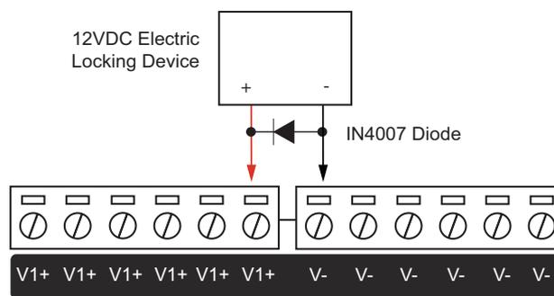
Note: The 1N4007 diode shown MUST be installed across the + and - terminals of any inductive load such as electric locks, magnetic or motorized devices.
